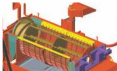
AXIAL FLOW THRESHING SYSTEM
